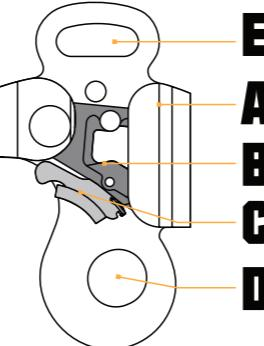
**EN:** (A) Body in aluminium alloy, (B) Steel toothed cam, (C) Safety device for the toothed cam in aluminium alloy, (D) opening for the connection to the bottom harness, (E) opening for the connection to the chest piece.
