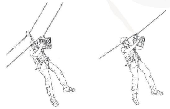
Note: During the process of traversing horizontally or inclinedly, the angle of the working rope shall be less than 150°.
