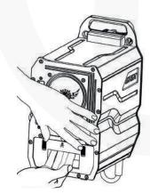
Up on battery mounting, verify that the battery is locked by battery lock and cannot be pulled out. Then turn the secondary lock to let the arrow upward, by which the secondary lock is locked.
