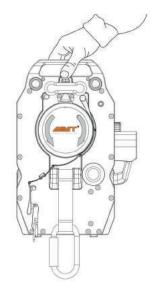
5.1.1.2 Make a loop on the rope, press the guide block by one hand, and by the other hand, pass the rope loop through the guide block and rope separator inside of the U-shaped fender, and reeve the rope on the rope sheave and tension it.
