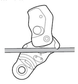
• Ensure CAPTO moves freely towards the anchor, and grabs the rope when pulled away from the anchor.
